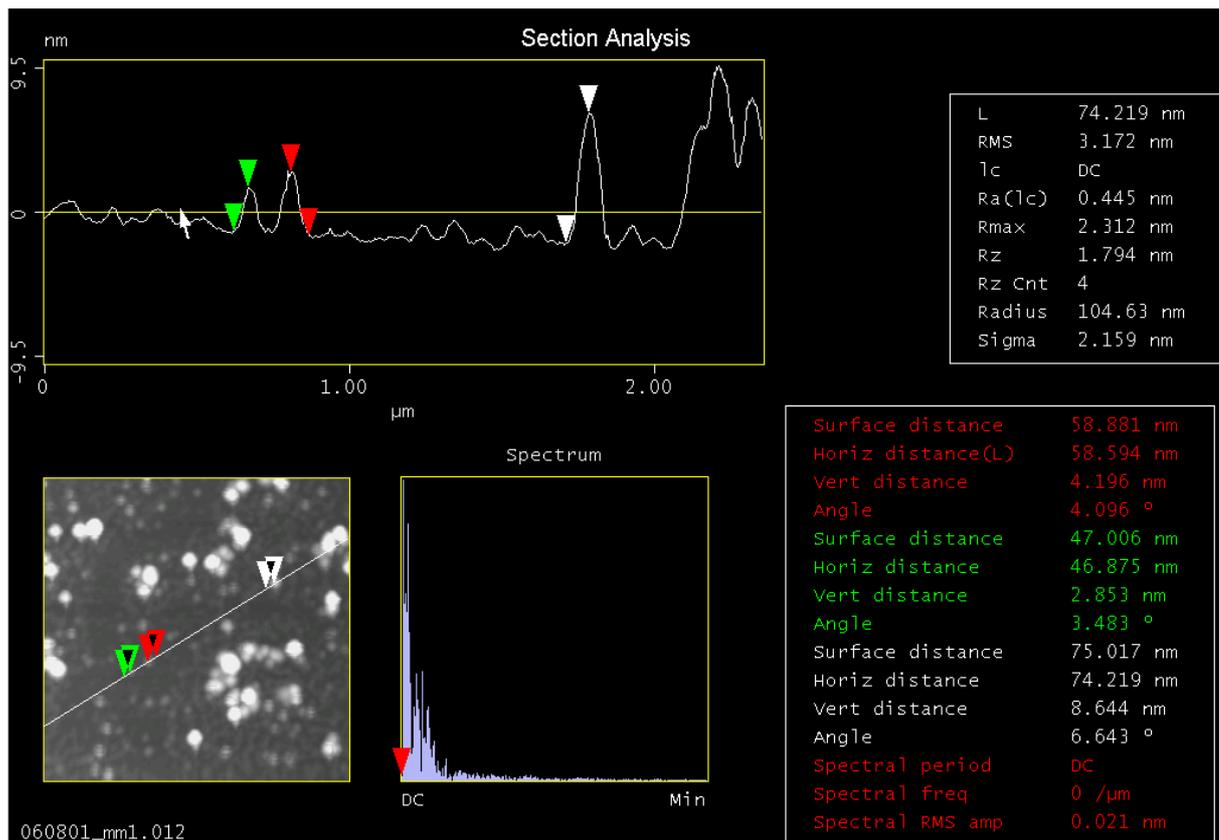
**Figure 20.** AFM section analysis of Concept Alkyd Figure 7. The area analysed is 2x2 µm large.
