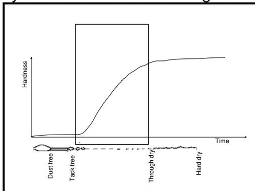
**Figure 1.** Typical alkyd binder drying process
