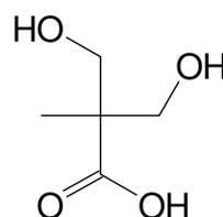
**Figure 13.** BisMPA (Di-methylol propionic acid)
