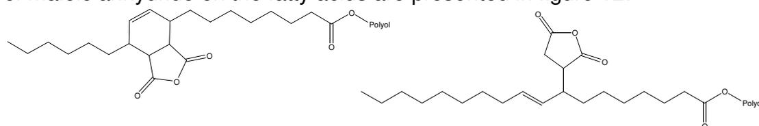
**Figure 12.** Dendritical fatty acid moieties modified with maleic anhydride for further molecular weight enhancement.
