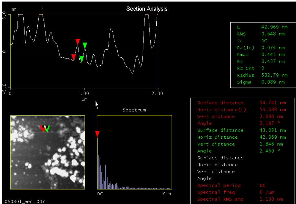
**Figure 18:** AFM section analysis of Concept Alkyd Figure 7. The area analysed is 2x2 μm large.
