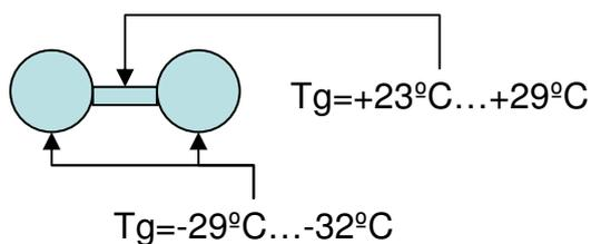
**Figure 7.** Dendritical moieties shielding a hard segment
