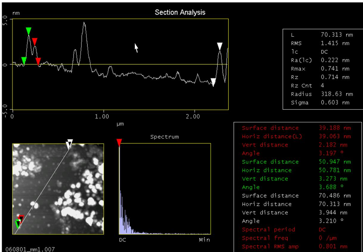
**Figure 19:** AFM section analysis of Concept Alkyd Figure 7. The area analysed is 2x2 μm large.
