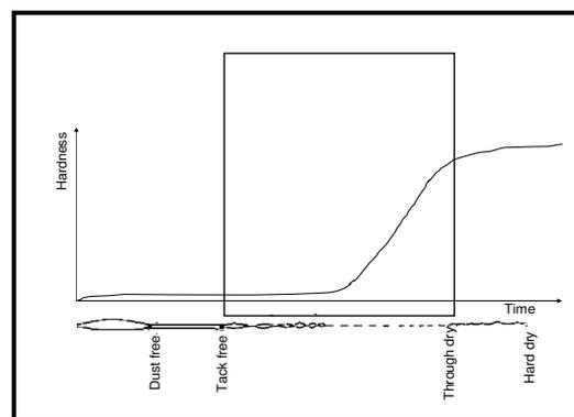
**Figure 2.** High Solids binder drying process
