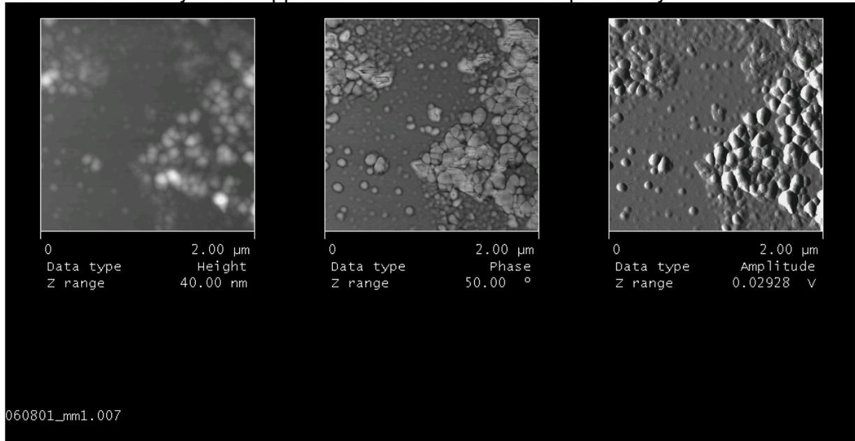
**Figure 16.** AFM image Concept Alkyd Figure 7. From left to right are representations of height, phase and amplitude.
