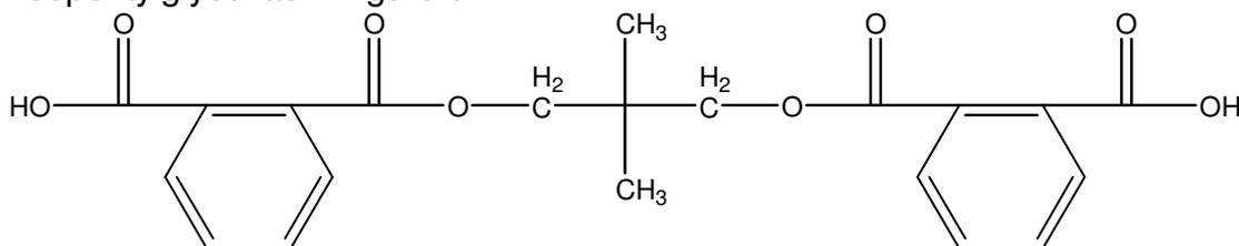
**Figure 9.** Hard segment obtained by reacting Neopentylglycol with Phthalic anhydride
