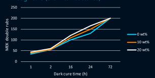
Curalite™ Ox has been formulated with cycloaliphatic epoxy and cationic photoinitiator and cured with a Hg lamp
