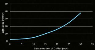
Curalite™ OxPlus has been formulated with cycloaliphatic epoxy and cationic photoinitiator, and cured with a Hg lamp
